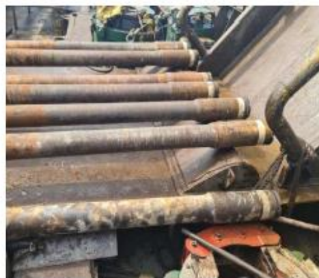
Drill pipe shown rolled off catwalk (note lack of pipe stop ramp side rail)
